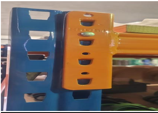
Interlocking beams and frames
