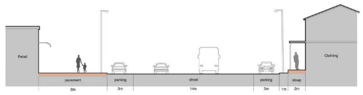
Figure 7. Voortrekker Street Commercial Core - Existing Cross Section
